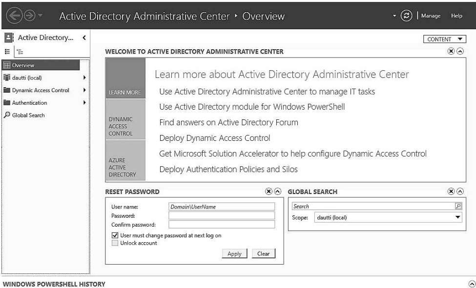
Rysunek 4.2. Active Directory Administrative Center w systemie Windows Server 2025
