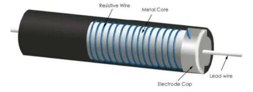
Figure 1.2: Wire-wound resistor
