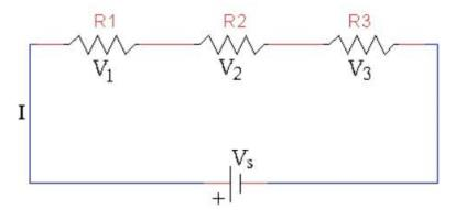
Figure 1.10: Series resistors
