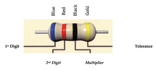
Figure 1.9: Sample resistor
