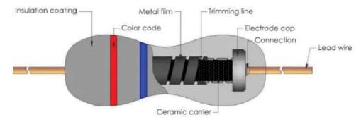
Figure 1.4: Metal film resistor
