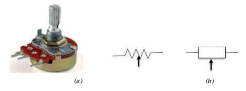
Figure 1.7: (a) Potentiometer and (b) symbol
