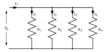
Figure 1.11: Parallel resistors
