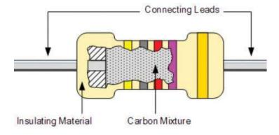
Figure 1.3: Carbon compound resistor
