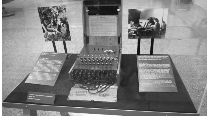
Figure 1.1: A photograph of an actual Enigma machine from World War II: From the author's personal collection
