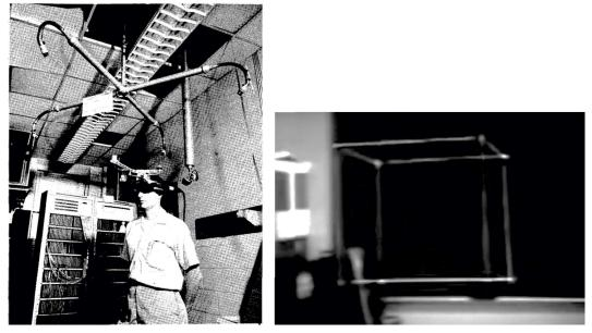
*Figure 1.3:* The first head-mounted display and how a 3D object can be seen through it. (*Ref:* Fall Joint Computer Conference Journal, 1968)
